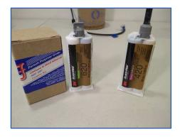
13. Install a mixing tip on the epoxy or urethane cartridge (mixing tips greatly reduce the amount of bubbles). Discard the first 1-2 ml of epoxy or urethane that comes out of the mixing tip. Insert the mixing tip deep into the syringe and inject the epoxy or urethane into the syringe. Try to fill the syringe without getting any air bubbles into the epoxy or urethane.
