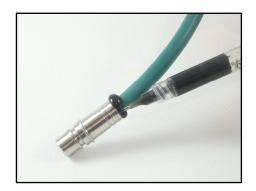
15. Clean off the excess epoxy or urethane with a paper towel and acetone or alcohol.
