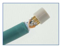
6. Abrade the last 3 cm of the cable jacket with sandpaper and clean with acetone to prepare it for potting. From this point on, be careful to keep this part of the cable jacket clean.
