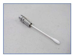
3. Slide the Locking Sleeve onto the cable with the internally threaded part of the Locking Sleeve facing towards the end of the cable. Then slide the Connector Shell over the cable. The end of the Connector Shell that has the flat surface should be facing the end of the cable. Secure the Locking Sleeve and Connector Shell with tape to keep them in place during the rest of the process.
